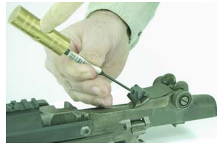
3. Drive roll pin flush.
