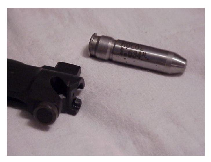
3) place the gauge in the bolt face, and into the chamber (differs for each firearm, a Mauser can actually strip the gauge out of the mag if you wanted, a Garand has to have it held on there until the bolt is closed). NOTE, you are closing the bolt with hand pressure only, NO OP ROD or SPRING is used to close anything, you removed them, right? Picture shows closing the stripped M1A bolt on the gauge using light finger pressure...
