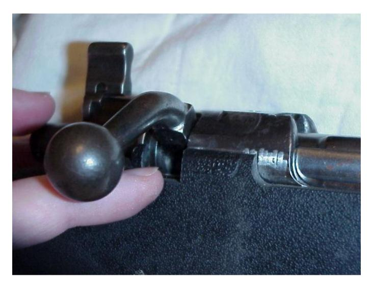
In the pictures, the M1A (with stripped bolt) closes on the "go" gauge, but will not close on the "no-go" gauge. Note the use of "two finger" pressure only on the bolt. The Mauser shown closed on the "go" gauge, and would JUST CLOSE ON NO-GO WITH GAUGE CONTACT. There was slight resistance. The actual picture shows contact using the .308 field gauge in this Israeli 7.62 conversion barrel...
