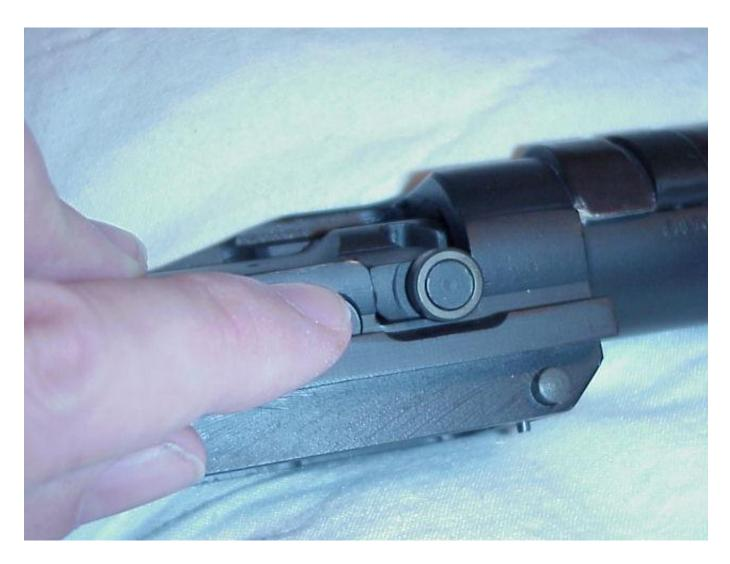
5) select the next gauge (normally, go, no go, then field), repeat number 4 above. You are looking for the gauge that won't allow the bolt to close with light pressure applied. In the M1A below, this is the "no-go" gauge.
