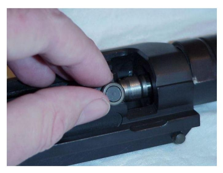
4) gently close the bolt on the gauge. I use two finger pressure. When the gauge touches the chamber end, and you feel it, you have measured the headspace! This is like using the calipers or the micrometer in shop, as soon as it touches, you are done! IF the bolt CLOSES WITH NO RESISTANCE on the first gauge, keep going. That gauge is too short to measure the headspace... M1A bolt closes on "go" gauge, below...
