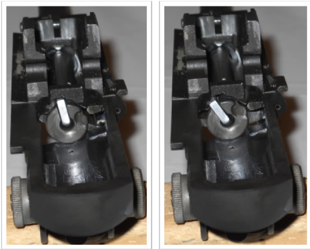
Left image: bolt fully engaged; firing pin free to strike the primer. Right image: bolt fully forward but not engaged; firing pin blocked by the safety bridge.
