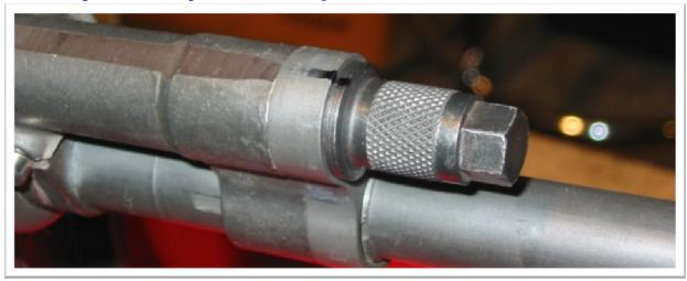
The gas components pictured have just under 700 rounds through them and they cleaned up very nicely. It was a USGI gas system with a Sadlak TiN gas piston (no groove). YMMV
