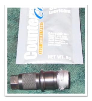
Using your gas cylinder wrench and tool of choice, torque the gas plug to match the witness mark you made before you disassembled the gas system. If you are using a torque wrench, the minimum recommended torque is 120 inch pounds (10 foot pounds) and the maximum is approximately 23 foot pounds. The popular ranges are 120 inch pounds to 150 inch pounds. Gas plug torque may affect accuracy so play around with what torque works best in your rifle. German torque is also acceptable (Good-N-Tight).
