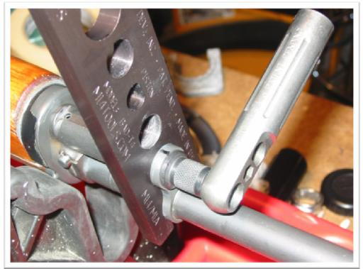
If you have the BAD-T4 gas cylinder wrench, ensure the threads are clean on your gas plug and screw it into the BAD-T4 wrench as pictured. This will give the plug a nice handle when cleaning and will also prevent it from rolling around on the bench.
