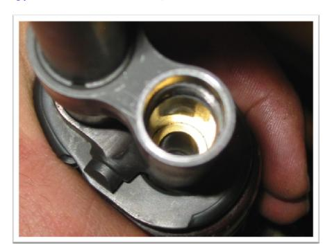
Ensure the threads of the gas plug are thoroughly cleaned and dry. Apply some anti-seize to the threads.
