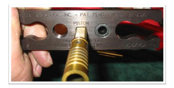
Next, clean the inside of the gas piston with a letter P and number 15 drill bits. You use the drill bits to scrape carbon from the inside walls of the piston. Lots of black dust will come out. This is normal.
