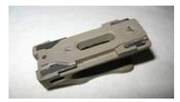
Check alignment again and load up your counter sink or 3/8" bit. If the alignment is off you can steer the countersink/drill bit around to center the hole. Just be patient and go slow. Be sure to countersink the TOP of the floor plate (little tab at the rear should be up when countersinking). Take just a little off at a time checking the screw heads to make sure they don't go through the holes. Stop when the heads are flush or close to it.
