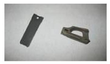
Using the tip of your utility knife (with a new blade I hope) lightly stab into the mount surface of the ranger plate to find out where the stainless steel backing plate is under the rubber and mark where you plan to drill.
